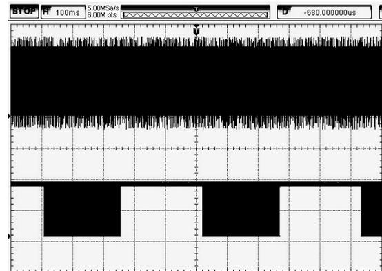
Fig. 2. Packet dropout when transmitted data is continuous (top: Original Signal, bottom: Received Signal)
