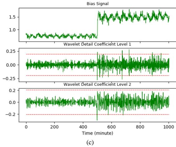
Fig. 4. MODWT and threshold setting of three example signals: (a) spike signal; (b) erratic signal; and (c) bias signal.
