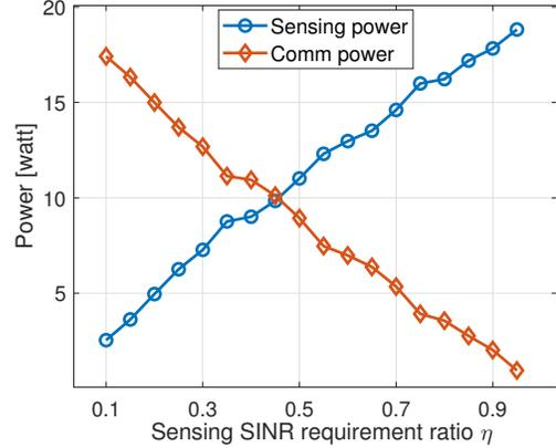
Fig. 4: Radar sensing power vs. Communication power [Watt]
