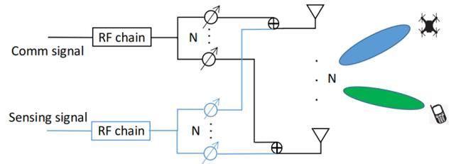
Fig. 1: Integrated MIMO radar and communication system
