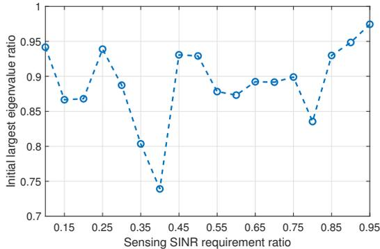
Fig. 3: Initial ratio  $\lambda_{\max}(\mathbf{X}^{(0)})/\text{Tr}(\mathbf{X}^{(0)})$
